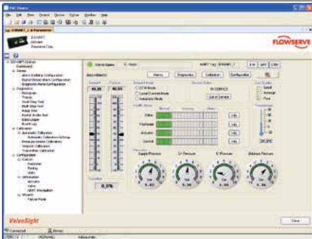
ValveSight™ displays green health bars indicating normal conditions of valve, actuator, positioner and process signals.
