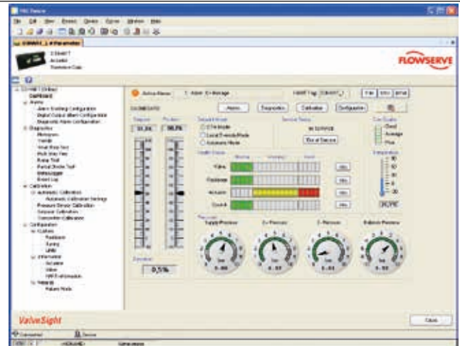
ValveSight™ has detected an issue, initially yellow bar starts to grow as it warns of an emerging problem thus providing early heads up that maintenance is recommended to avoid unplanned stoppage, then when alarm limit is reached an alarm is generated – red bar in picture indicates ValveSight has sent an alarm to the control system of the plant.
